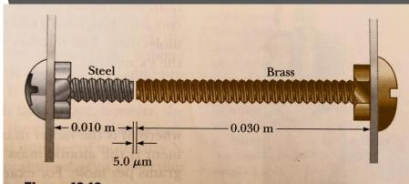
**Figure 18.10** (Example 18.3) Two bolts attached to different parts of an electrical device are almost touching when the temperature is 27°C. As the temperature increases, the ends of the bolts move toward each other.
